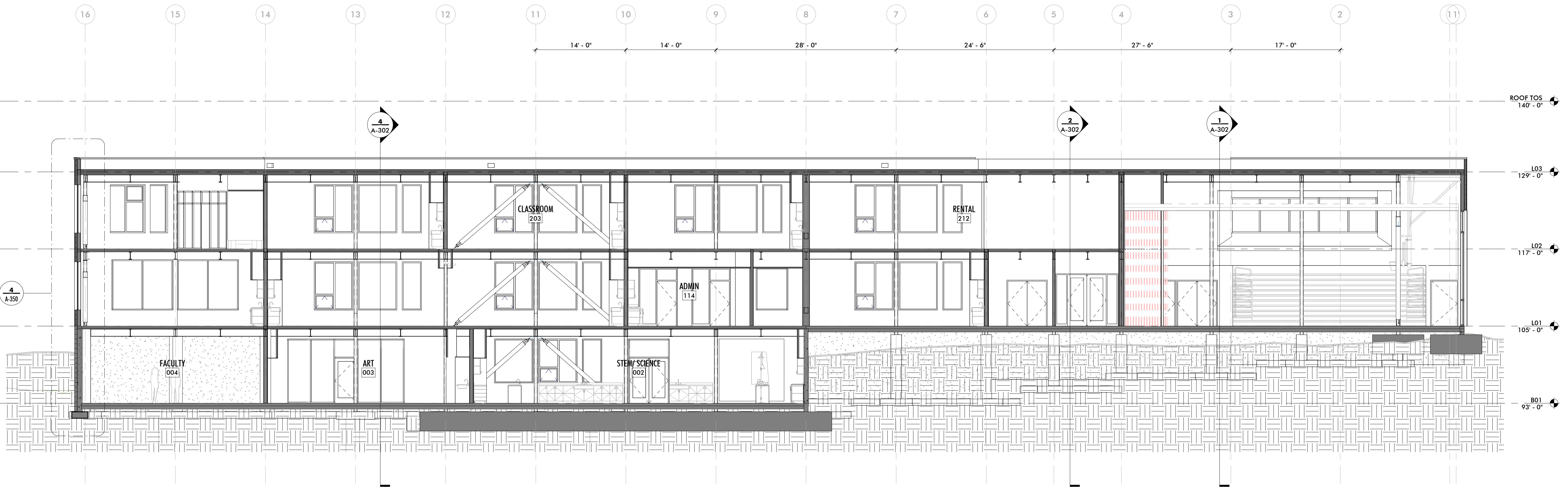
2 EAST-WEST SECTION THRU MULTIPURPOSE 1/8" = 1'-0"
